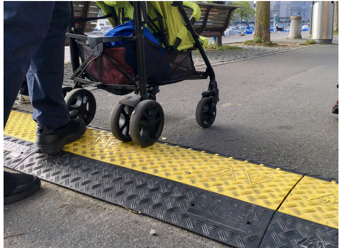
Cable crossover in Zurich
